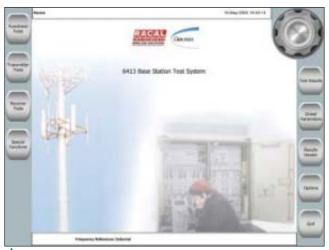
Fig. 1 The front panel display utilizing touch-screen controls.
