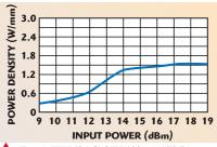
ightharpoonup Fig. 1 HVMSAG CW 468  $\mu$ m FET power density performance at  $V_d$  = 25 V and 3.5 GHz.
