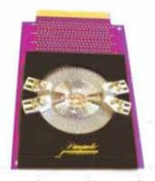
Our patented probe structures provide the precision and ruggedness you require for both production and characterization testing. And, only Picoprobe® offers the lowest loss, best match, low inductance power supplies, and current sources on a single probe card.
