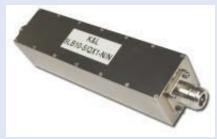
The model 9LB10-5/QX1-N/N is a lumped component filter designed for customers who have low frequency, high power requirements where low insertion loss is a must. This unit is versatile and works well in military and commercial environments. This filter offers < 2 dB insertion loss across 100 percent of passband. Other specifications include > 90 dB stopbands, 2.0 VSWR and 50 W CW power. Size:  $6.0" \times 1.5" \times 1.5"$  with type N connectors.
