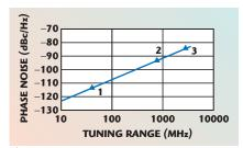
Fig. 11 Phase noise (at 100 kHz offset) vs. tuning range, using an external three-section filter.
