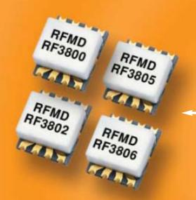
Optimized for base station transceiver and high-power amplifier applications, our RF3800 series of amplifier solutions keep people connected through high efficiency, high linearity, high gain and high power. Assembled in thermally enhanced AIN LCC-8 packages, our solutions offer a more robust alternative to lower power plastic packaged pre-driver amplifiers.
